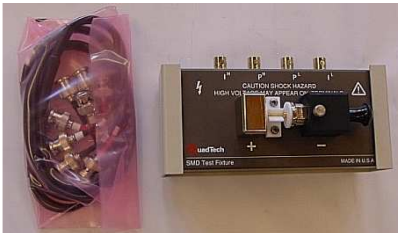
Figure 2-14: 7000-07 Low Voltage Chip Component Test Fixture
